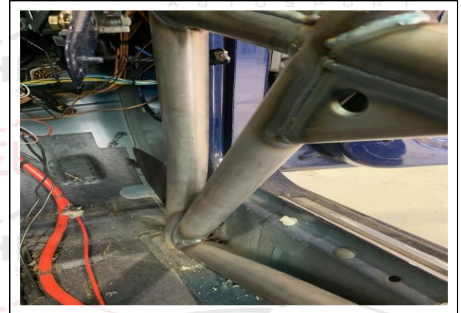
PHOTO 6 FRONT ROLLBAR TO FLOOR ATTACHMENT
