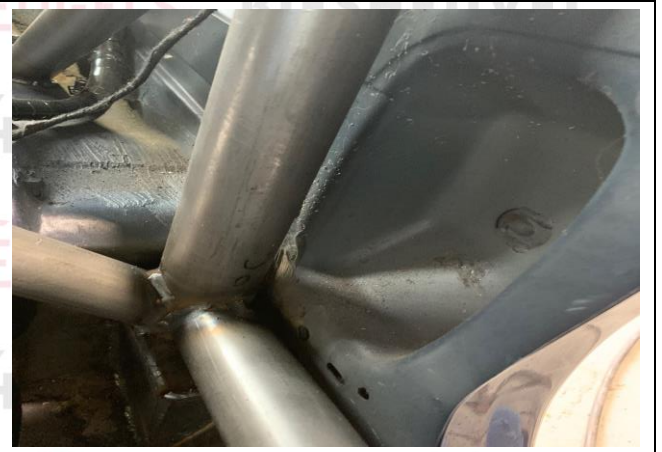
PHOTO 4 MAIN ROLLBAR TO FLOOR ATTACHMENT
