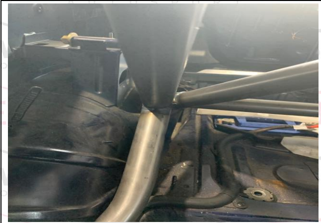
PHOTO 5 REAR BACKSTAY TO BODYSHELL ATTACHMENT
